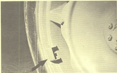
Figure 16. Valve stem protector
